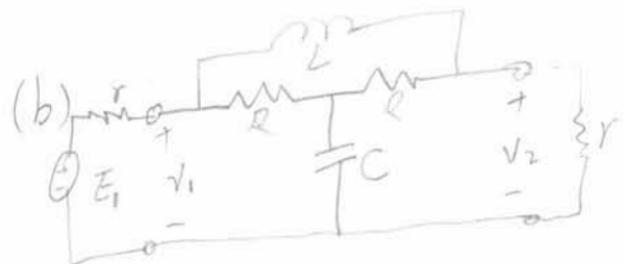
$$V_1 = \frac{E_1}{2} = Z_{11} \cdot \frac{E_1}{2r} - Z_{12} \frac{V_2}{r}$$
