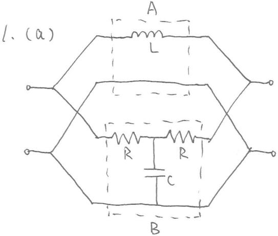
$$Y_A = \begin{bmatrix} \frac{1}{SL} & -\frac{1}{SL} \\ -\frac{1}{SL} & \frac{1}{SL} \end{bmatrix} \quad Y_B = \begin{bmatrix} \frac{SC + \frac{1}{R}}{SRC+2} & -\frac{1}{R} \frac{1}{SRC+2} \\ -\frac{1}{R} \frac{1}{SRC+2} & \frac{SC + \frac{1}{R}}{SRC+2} \end{bmatrix}$$
